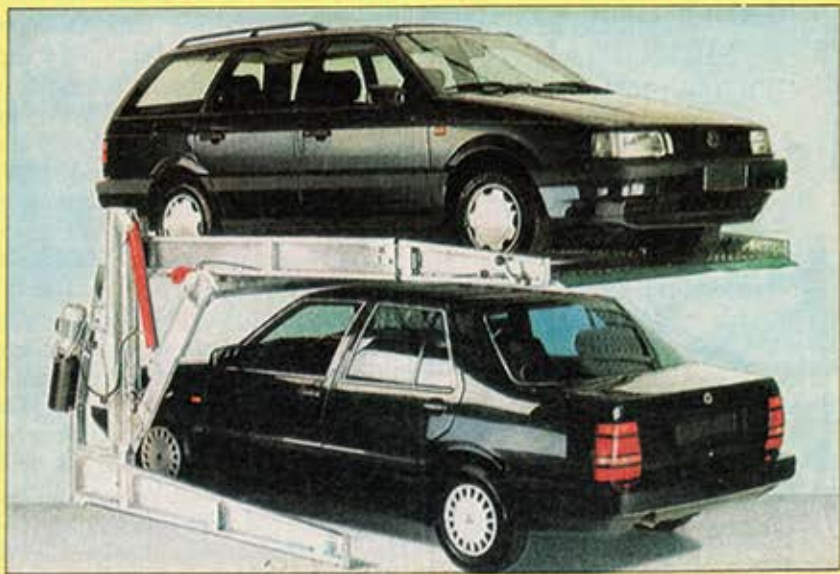
MECHANICAL CAR PARKING
