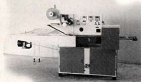
FORM FILL & SEAL MACHINE WITH BUCKET ELEVATOR & ELECTRONICS WEIGHERS FOR PACKING VARIOUS ITEMS. PHOTO CONTROL
