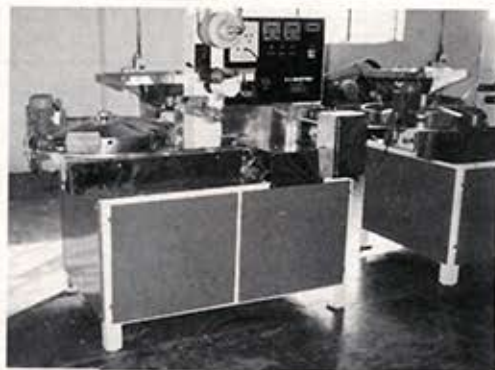
HORIZONTAL FLOW PACK WRAPPING MACHINE HIGH SPEED HARD BOILED CANDY WRAPPING MACHINE SPEED: UP TO 750 PACKS/MIN. PHOTO CONTROL
