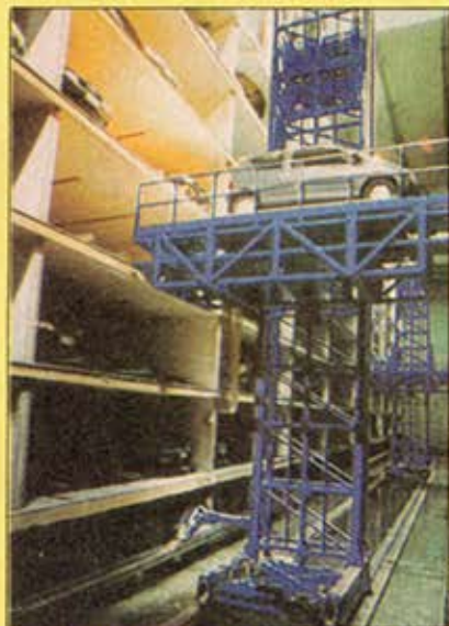
INTELLIGENT AUTOMATIC MECHANICAL CAR PARKING
