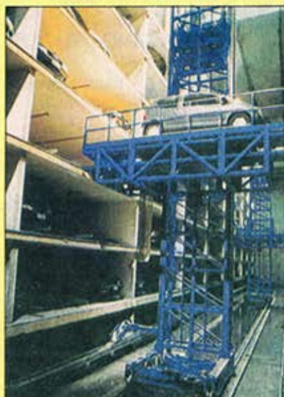
INTELLIGENT AUTOMATIC MECHANICAL CAR PARKING
